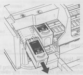
5 Unpack a new FINE Cartridge and remove the orange protective tape (A) gently.
